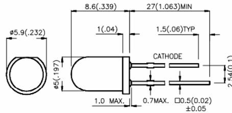
Note that the cathode can be identified by the shorter lead and also by the flat on the flange of the bulb.
