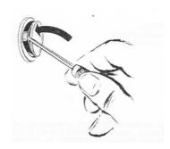
Slide a small flat-bladed screwdriver under the old tyre as shown. Slide the screwdriver round the wheel, levering the tyre over the edge until it is removed.
