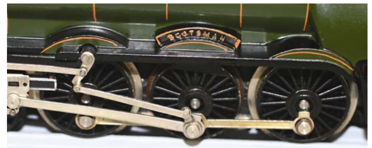
Open spoke wheels showing fluting on coupling rod
