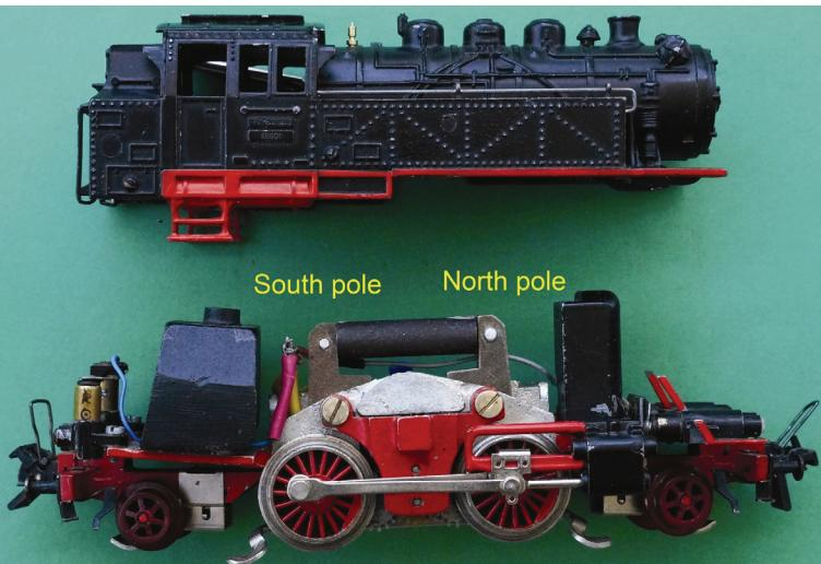
Both Franz and I routinely replace the weak 64 year old AlNiCo TRIX EXPRESS magnet shown above with a custom made NdFeB N45 magnet. These are the strongest commercially available permanent magnets; they are commonly, but somewhat incorrectly, known as 'Neodymium' magnets. The temperature at which the property of ferromagnetism spontaneously disappears is known as the Curie point; only three elements are ferromagnetic at room temperatures:- Iron, Nickel and Cobalt.
